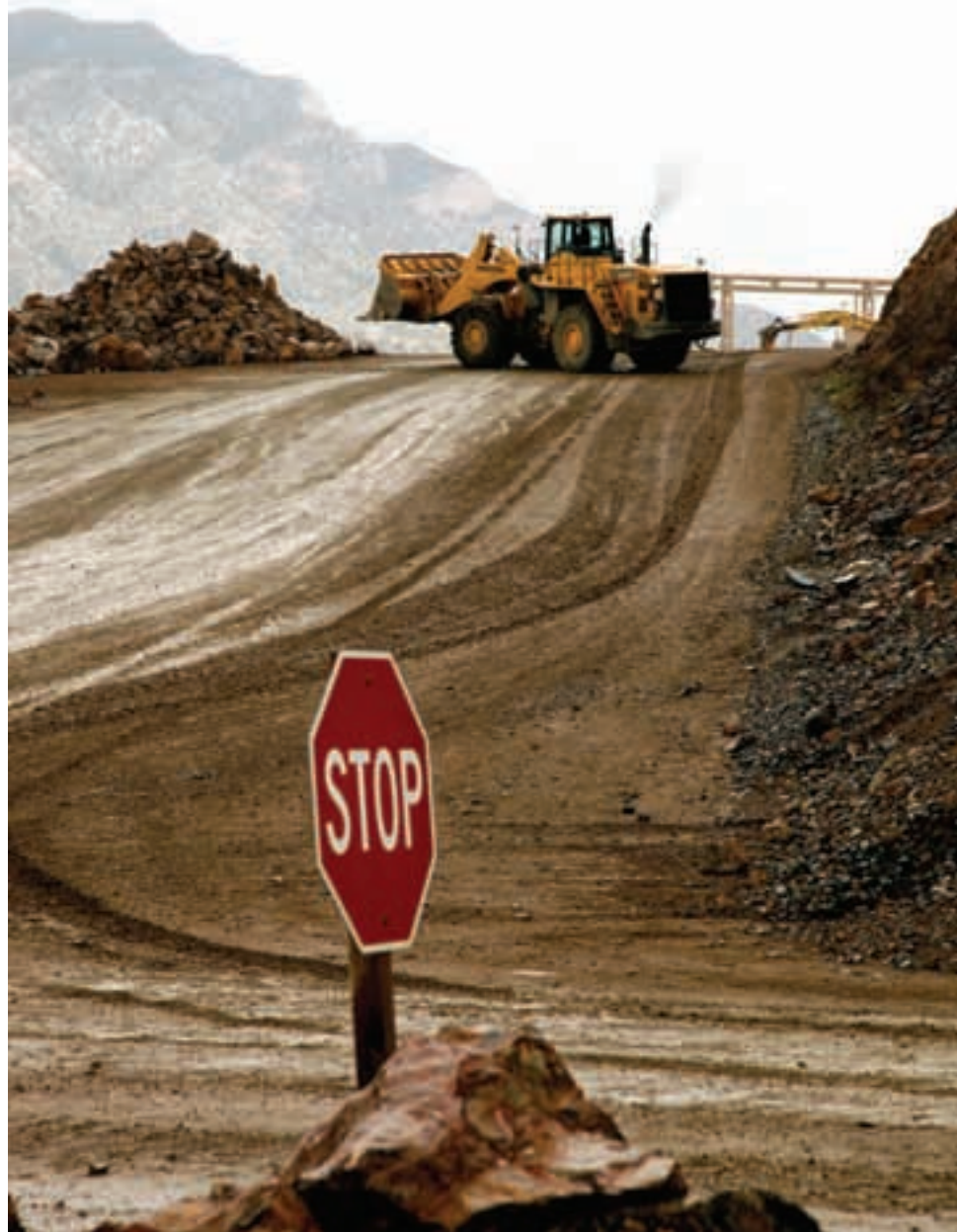
A front-end loader moves rocks from the pit at Mountain Pass Mine. JOHN GURZINSKI
